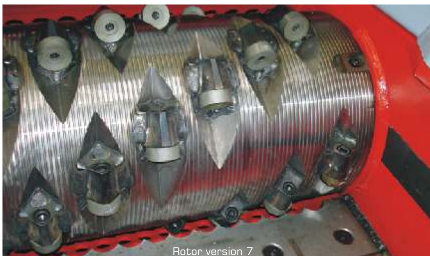
Concave cutting heads can be turned up to 4 times.
