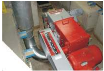
Shredding wood waste from a plate saw with an RHZ 400 S horizontal shredder set up below ground
