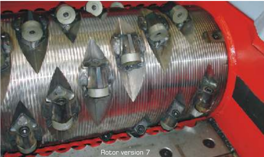
The highly efficient scissors cut out of the concave ground circular cutting heads enable a very high work rate with very little effort. The knives are mounted on a rotor and can be turned up to 8 times with just a few adjustments before having to be exchanged completely.
